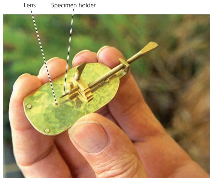
▲ Figure 1.2 Reproduction of Leeuwenhoek's microscope. This simple device is little more than a magnifying glass with screws for manipulating the specimen, yet with it, Leeuwenhoek changed the way we see our world. The lens, which is convex on both sides, is about the size of a pinhead. The objective to be viewed was mounted either directly on the specimen holder or inside a small glass tube, which was then mounted on the specimen holder.
